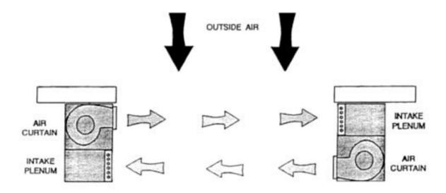
Based on the above figure, each air curtain device has an air inlet enclosure, which is precisely located opposite the linear valve of the opposing air curtain device. The functionality of this model is to create a thicker air curtain against the door. The velocity of the air emanating from this device will be lower compared to devices that are installed above the door. This model of the air curtain also has the capability to be fitted with a heating coil and a filter.
