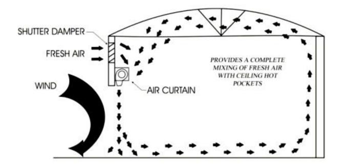
Fresh air enters through this damper and mixes with the stagnant air at the top of the building or hall, creating a state of equilibrium within the space. Naturally, under such conditions, the efficiency of the air curtain device will be enhanced.
