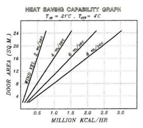
From the above graph, the amount of energy wasted is calculated as 1.35 million calories per hour for one year (four cold months).
