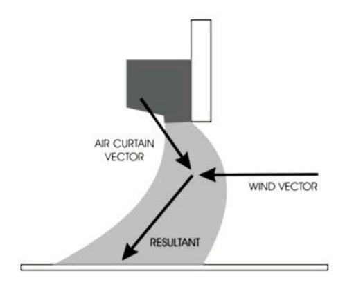
The air that is expelled from the Air Curtain device carries energy due to its high velocity and mass and is represented as a vector. Similarly, wind, which also possesses energy, is depicted as a vector at the doorway. The collision between these two vectors results in the formation of a third vector.
